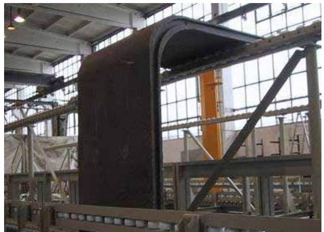
POLYCRETE® bend element for cladding a collector
